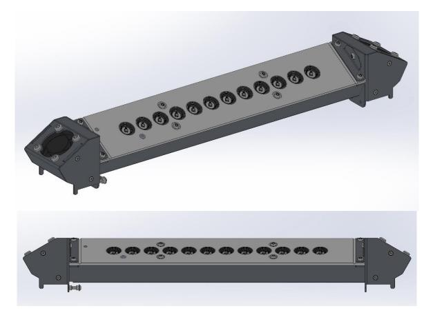
The device is a sustainable UV-C part of an application for disinfection of trays. The innovative design constructed on LED iBond's patented ACP framework provides a compact near-field UV-C LED kit optional for both retrofit and for new installations.
