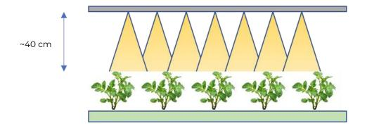
The panels can easily be placed higher than 40 cm above the crops (final height) but it will mean that an increased amount of light energy will be wasted and the PPFD measured at the crops will drop slightly.
