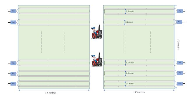
Illustration 1: Growth area with a size of 4.2x30 meters (two areas). Power supply units (PSU) are mounted at each side of the grow area for easy access and installation. The power supply units and electrical wiring are mounted directly on the suspended mounting rail system and will not interfere with crops.
