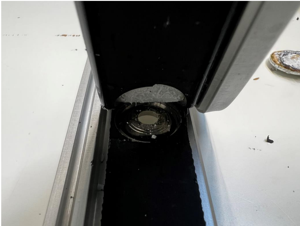
Photo 28 Visual inspection, IPX7. No ingress of water observed inside main enclosure.
