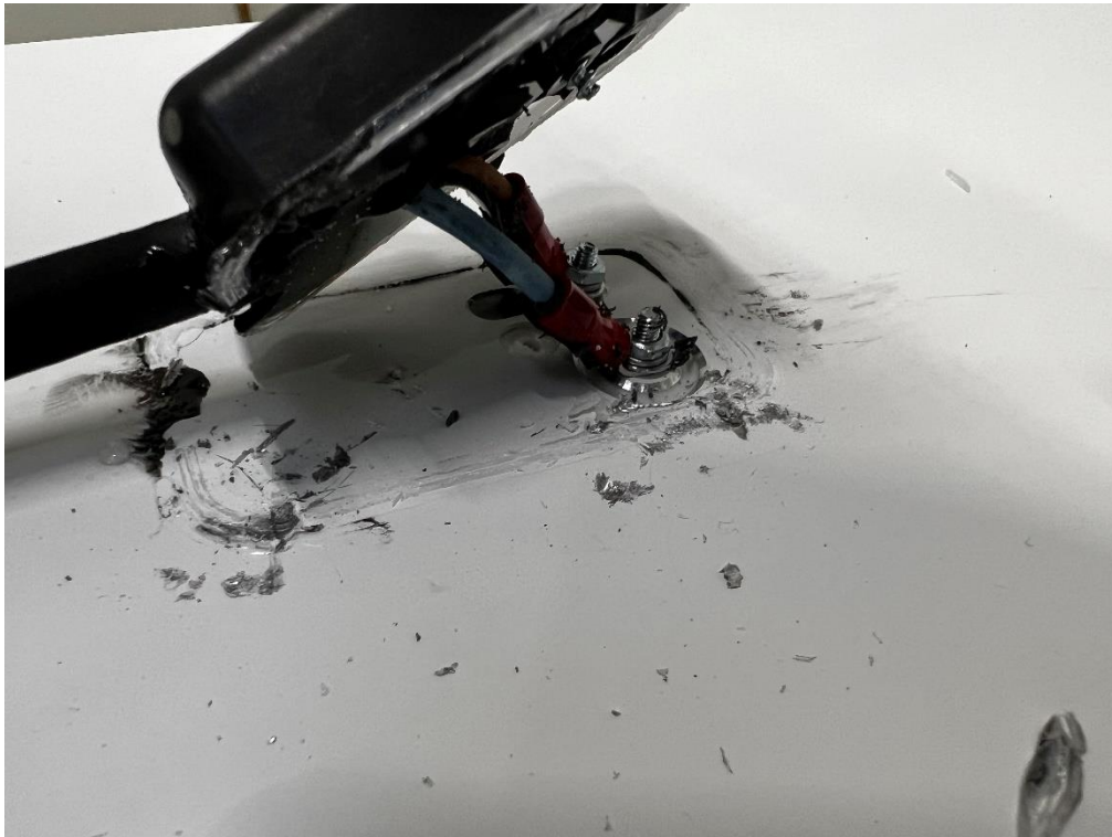
Photo 25 Visual inspection, IPX6. No ingress of water observed inside power connection.
