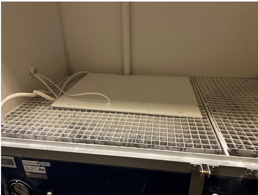
Photo 10 After exposure, IP6X.
