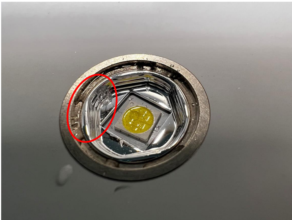
Photo 33 Visual inspection, IPX7. Ingres of water observed inside LED socket (numbered 1 on overview photo) – Lid removed. Similar when opening the sockets shown on photo 34 and 35.
