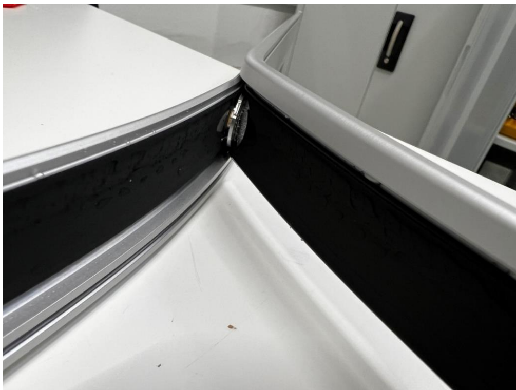
Photo 20 Visual inspection, IPX6. No ingress of water observed inside enclosure.
