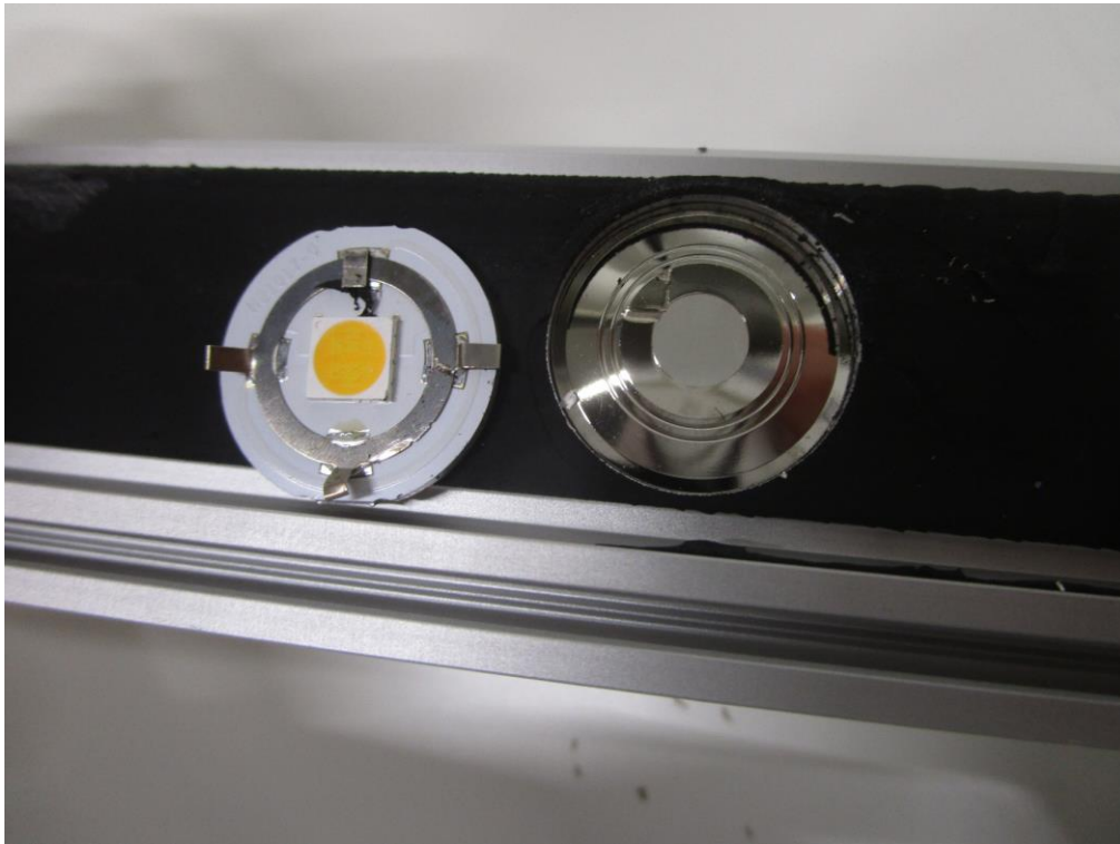
Photo 7 Visual inspection. IP6X. No dust observed inside main enclosure.
