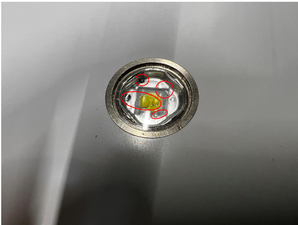
Photo 21 During exposure, IPX6.
