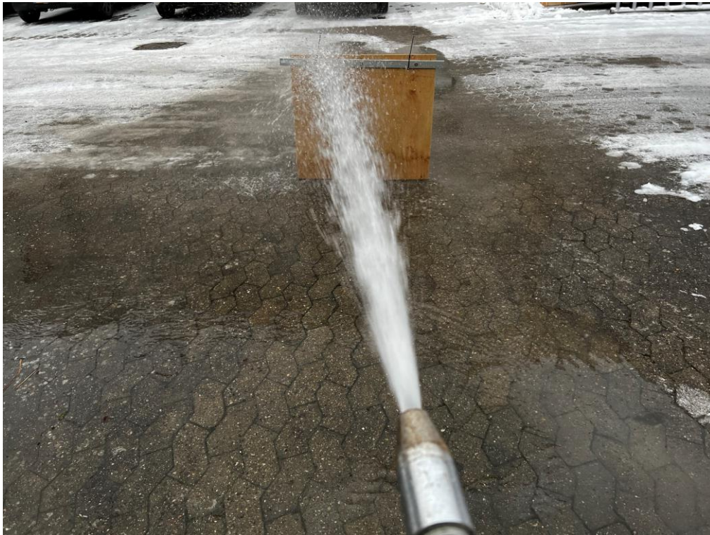
Photo 16 During exposure, IPX6.
