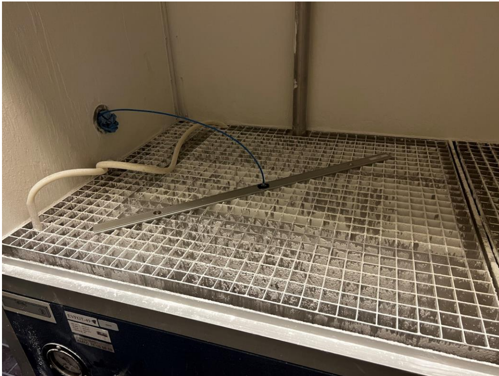
Photo 3 Before exposure, IP6X.
