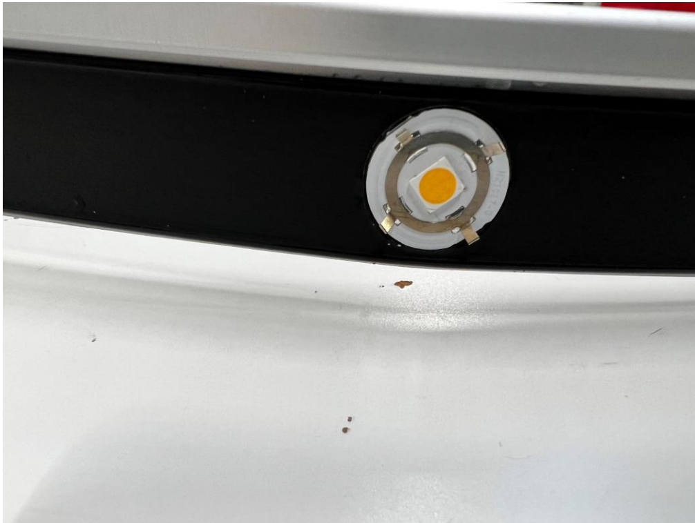
Photo 18 Visual inspection, IPX6. No ingress of water observed inside enclosure.
