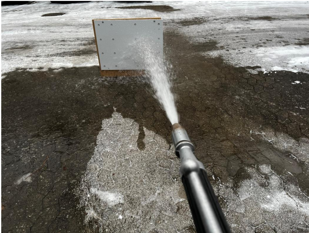
Photo 21 During exposure, IPX6.
