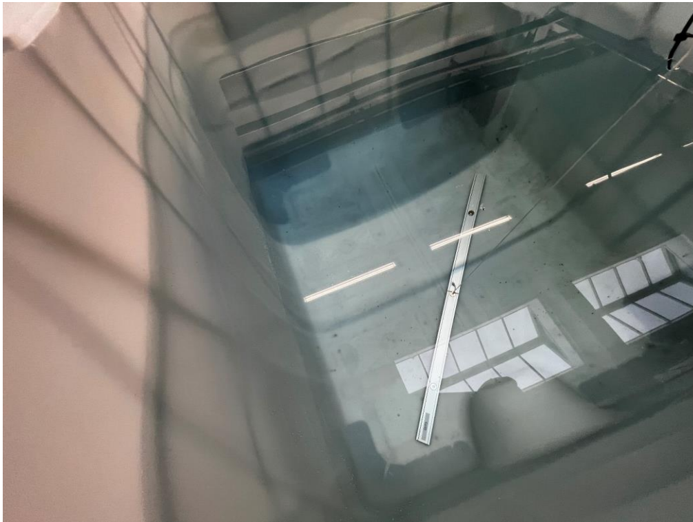
Photo 26 During exposure, IPX7.
