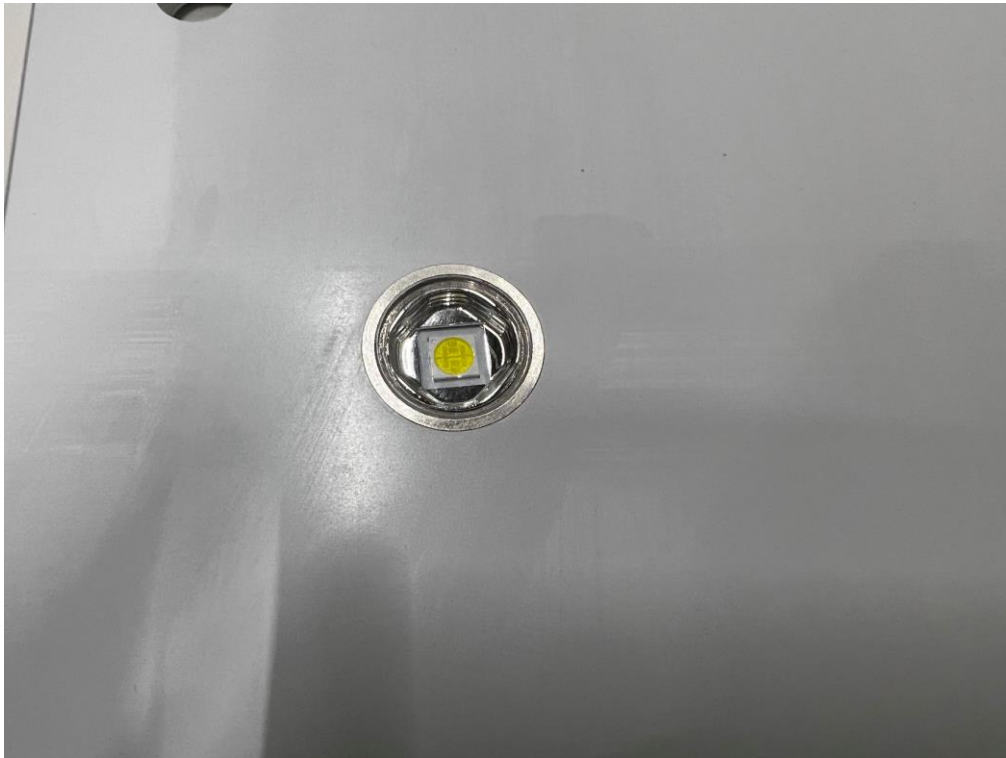
Photo 11 Visual inspection. IP6X. No dust observed inside LED sockets.
