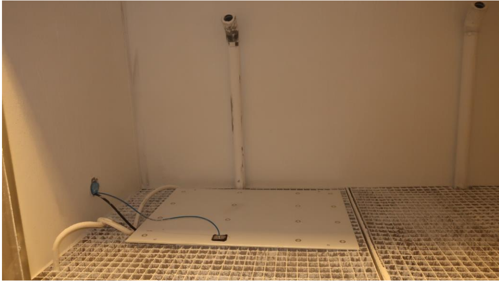
Photo 9 Before exposure, IP6X.
