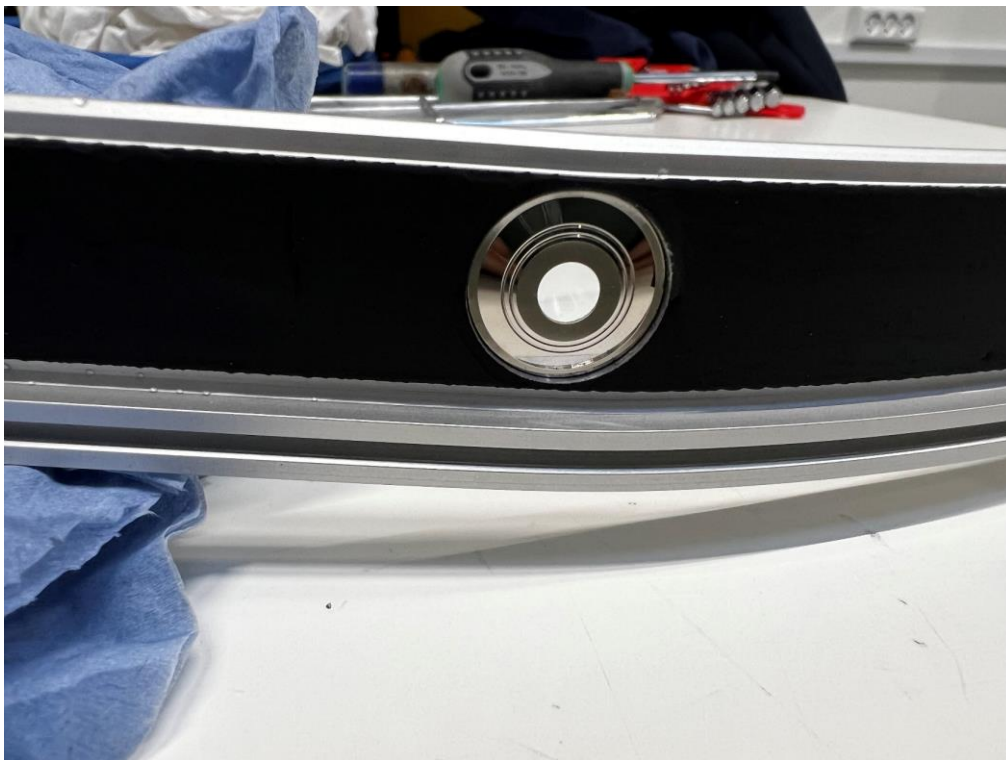
Photo 19 Visual inspection, IPX6. No ingress of water observed inside enclosure.
