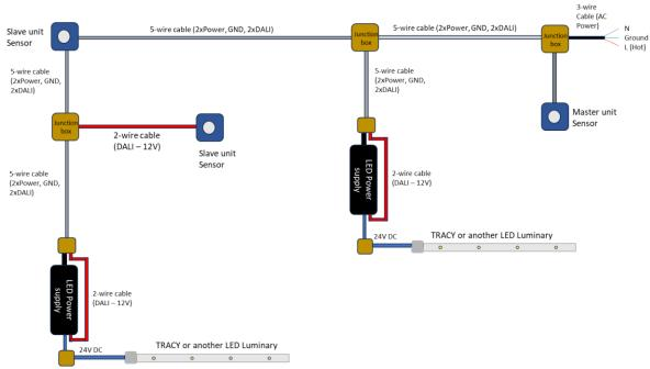
Below is an illustration of a distribution cabling network (example only).
