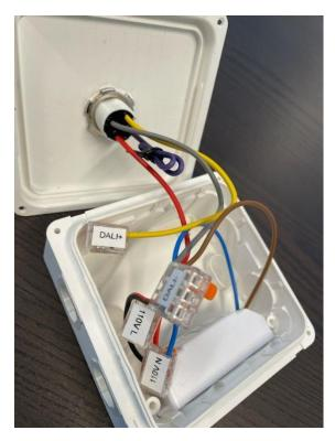
Figure 8 Interior of Master Unit Controller with DALI 12V DC power supply. Waga connectors for wiring.
