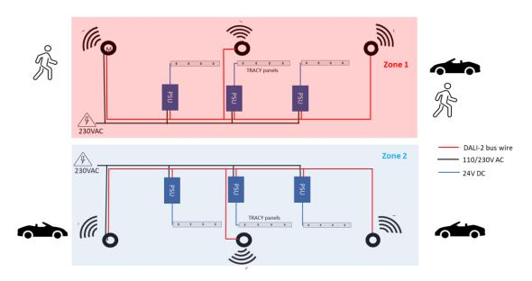
Figure 6 Electrical configuration of two zone solution - Example
