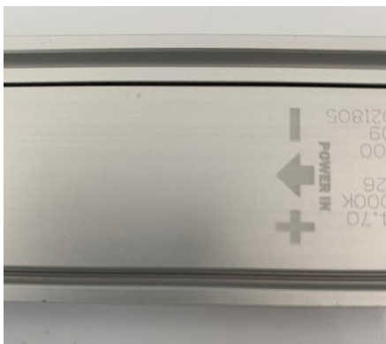
Figure 2 Label on backside of panel indicates polarity of each side of the panel.
